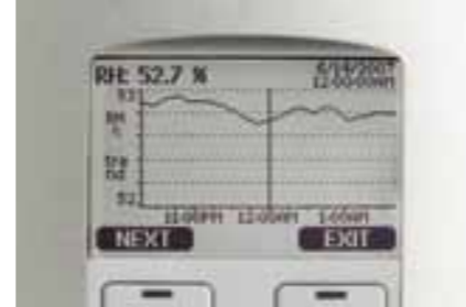
The display shows measurement trends and over four-year real time measurement history.
