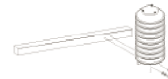
DTR502B horizontal beam installation.
