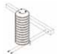
DTR503A horizontal beam installation.
