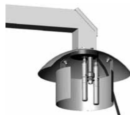
For calibration, a portable HMP77 reference probe is easy to attach beside the HMT337 or PTU307 probe.
