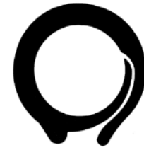
Stinger Cover Cross-Section
