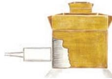
Content control of tablets in blister packages with capacitive sensors (KAS)
