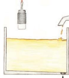
Overflow protection of casts, for example for plastic lenses for glasses with capacitive sensors of the KXS-Extreme series.
