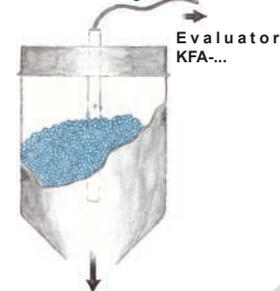
Level control of different rod media with TRUE- or PER Level rod probes with connection head (KFX)
