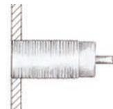
The **non-flush** mountable sensors are designed for applications, in which the medium to be monitored comes in direct contact with the sensor. In such level monitoring systems, the sensor head is completely immersed in the powder, granulate or liquid.
