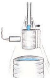
Capacitive sensors of the KXS-Extreme-series operate on the basis of the three-electrode principle. With this measuring principle, one electrode is removed to the outside. The protective conductor-potential PE - i. e. the machine and system potential - is now also used as a measurement electrode. The evaluation takes place with remote electronics.
