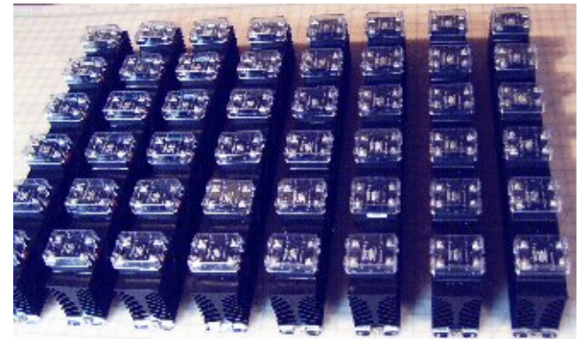
Eight "6-packs" with Power-io's HDD-6V15 IGBT hockey pucks = high speed PWM switching of 600 VDC and up to 720 total amps in a 30 x 23 inch area.
