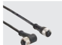
Female connector M8 and M12 - Self-locking vibration-damping ring nut. - High flexibility wire suitable to be used in movable chains - Protection degree IP68 - Gold plated contact (resistance < 5 mΩ) - Connector body in polyurethane
