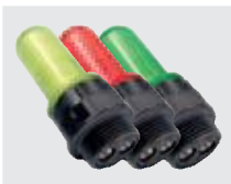
Light indicators A light indicator is used in order to visualize a change of state of the electric contacts inside the switch. It can be installed only in the series FL, FX, FZ or FS by screwing it on one of the conduit entries not used for electric cables. Protection degree IP67.
