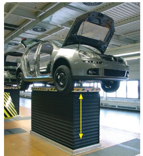
Draw-wire sensors monitor the height of lifting platforms on automobile production lines.
