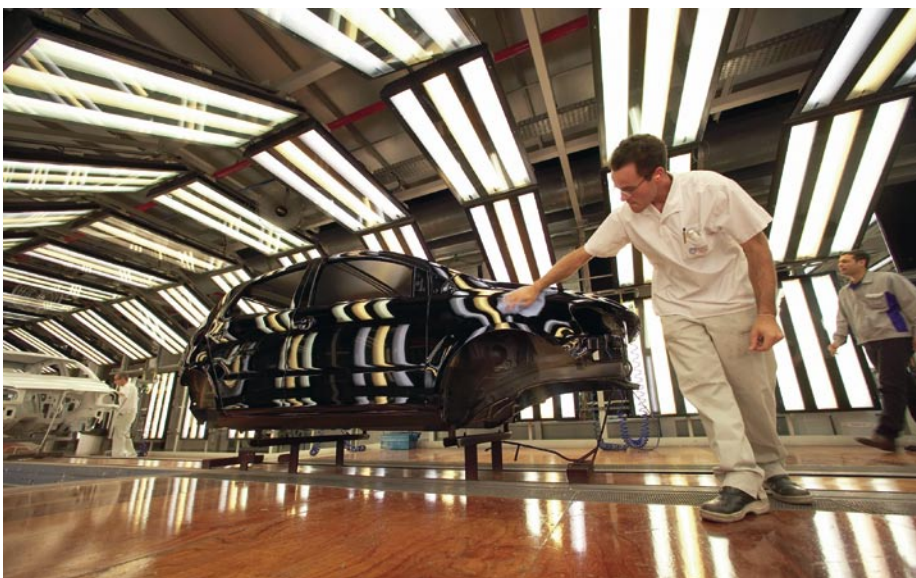
Previous visual inspections are replaced by the completely automatic reflectCONTROL.
