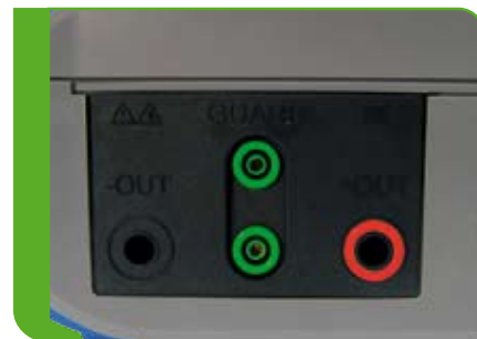
Guard terminal for connecting shielded test leads
