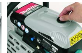
Bayonet lock for easy removal of filter compartment lid without tools.
