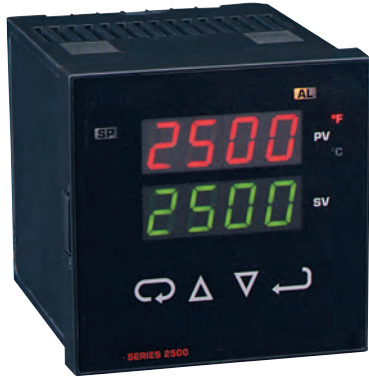
Panel cutout 3.622" x 3.622" (92 x 92 mm). Depth Behind Mounting Surface: 4" (103 mm).
