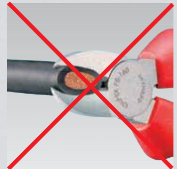
Cut performed with a Diagonal Cutter: high effort required, inaccurate cut, considerable deforming and crushing of the cable
