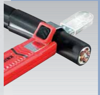
Self-turning drag blade for comfortable dismantling
