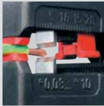
Precise stripping prevents damage to the conductor
