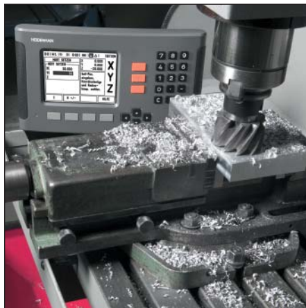
Position display on a milling machine
