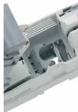
busbar cover closes automatically when switch operating cover with inserted fuse-link is closed
