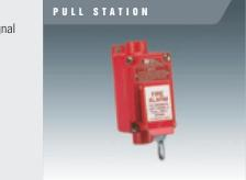
Explosion Proof pull station activates emergency equipment, signals or alarms from within a hazardous environment. Rated for Class 1, Division 1 applications. The two step activation includes a swing up front cover to expose the pull ring which activates the alarm; this two step process prevents accidental activation.
