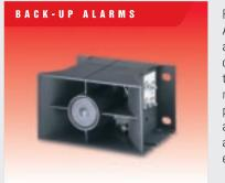
Federal Signal's Model 253 Back Up Alarm samples ambient noise levels and adjusts sound output automatically, providing just the right output to signal an approaching forklift, tow motor, dump truck, tractor or general purpose vehicle. Completely sealed against moisture and dust, these alarms are suitable for use in any environment.
