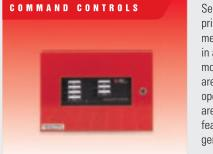
SelecTone® Command Units provide prioritized tones, pre-recorded voice messages, music and public address in any SelecTone system. Wall mount, rack mount and desktop units are available in 24VDC or 120VAC operating voltages. Command units are the basis of simple yet full featured plant communication and general alarm systems.
