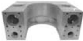
800 pound, integrated circuit manifold with DIN Cartridge logic for counterbalance and 1000 GPM regen capabilities.
