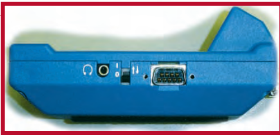
Headphone jack, on-off switch, and serial port for downloading to a PC.
