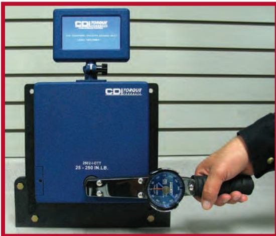
Perfect for checking dial torque wrenches.
