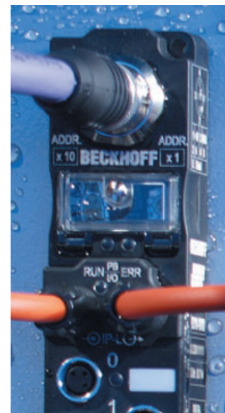
IP-Link interface on the Coupler Box for the connection of up to 120 extension modules
