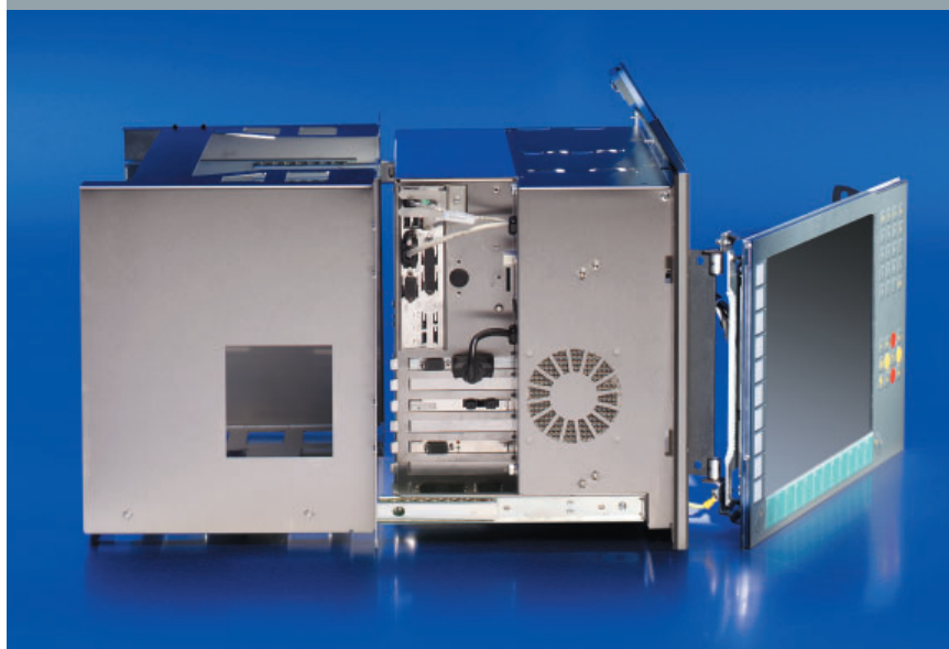
The mounting frame for withdrawal of the PC allows it to be mounted from the front. Connection cables are accessible from the side, as soon as the computer core slides out.
