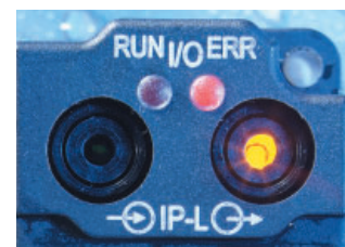
IP-Link interface on the Extension Box for communication with the fieldbus coupler
