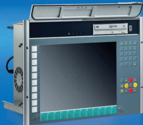
The CD/DVD drive is accessible under the lockable front flap.
