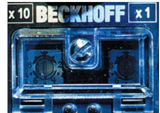
Programming interface under hinged inspection window
