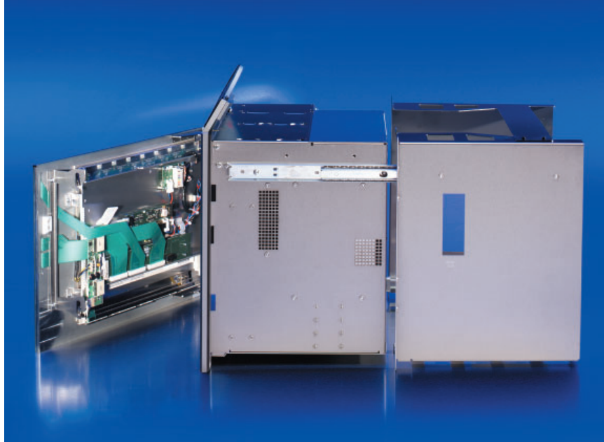
The mounting frame for withdrawal of the PC allows it to be mounted from the front. Connection cables are accessible from the side, as soon as the computer core slides out.
